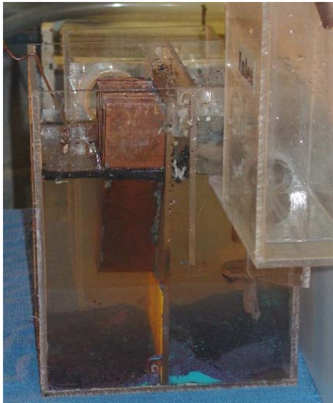
Figure 3. Photographs of the model of the TERRE KLEEN device. Sediment storage provided in both the catch basin for larger particles, trash and other debris, and below the inclined cell settlers for sediment removed by the inclined cells.
